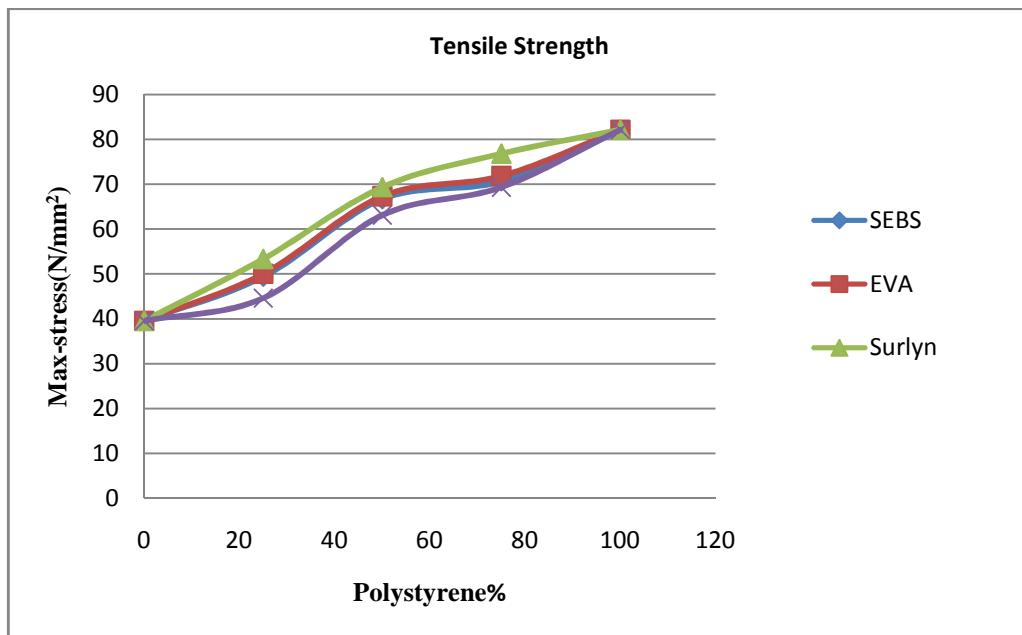
**Figure 1: Tensile Strength at Different Compatibilizers (5% w/w) and Different PS/PP Compositions**
